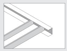
1: Mark the horizontal ceiling at the required height on all adjoining walls. Mark the lower side of the U-profile and fix it to the wall using 6 mm dowels in predrilled holes. Determine and mark the anchor points for the C60 profiles. Always install the first adjustable suspension bracket max. 300 mm from the wall.
