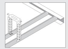
2: Hold a main profile with the opening facing upwards and screw on the adjustable suspension bracket to the side of the profile at the desired height. Bend back any excess section of the adjustable suspension bracket. Assemble the main profiles longitudinally using C-connectors, and terminate the main profiles in the U-profile.
